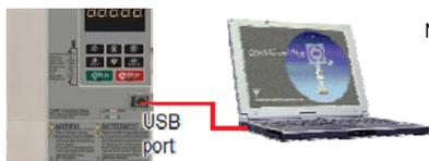
Note: Users can also use the WV103 cable included with earlier Yaskawa models. Simply remove the operator keypad to access the comm. port.
