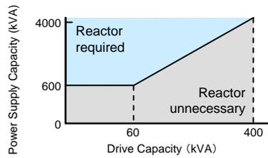
Note: Reactor recommended for power supplies larger than 600 kVA.
